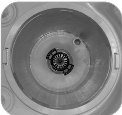
**Step 3:** Remove the E-Z Lock Filter Screen by inserting the tip of a flat-blade screwdriver into the slot of the E-Z Lock Filter Screen as shown and gently apply outward pressure until that catch releases. Then lift to remove.
